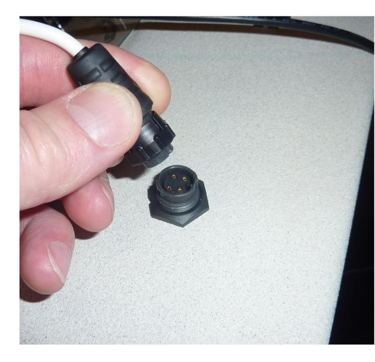
After inserting the plug, turn the collar on the plug clockwise to lock the plug into position.
