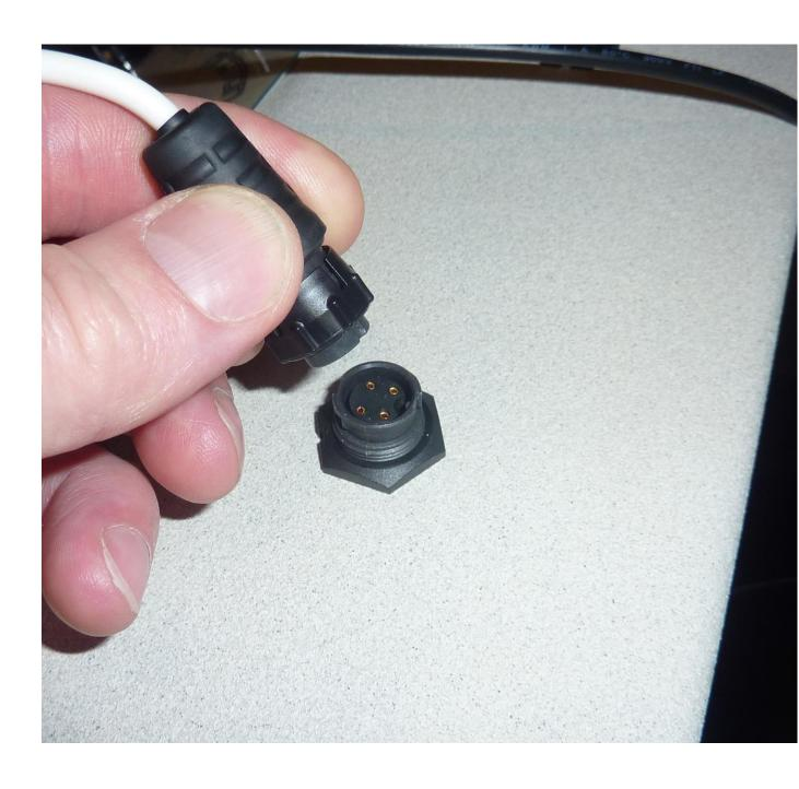
After inserting the plug, turn the collar on the plug clockwise to lock the plug into position.
