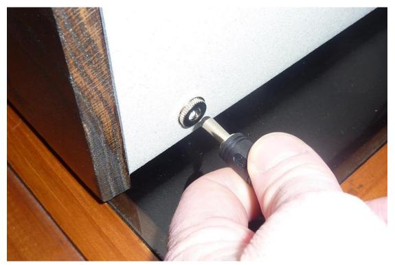
The Radio Frequency Sound Probe (RF Sound Probe, or RFSP for short) plugs into the headphone-style jack on the right, labelled "RF Sound Probe" (see below).
